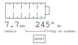
A Reset button is only available when the User controlled counter is displayed or if counter includes energy from a previous drive. The portion of the energy accumulated in the energy counter from the current drive is always protected and cannot be cleared while driving. If no trip is active then pressing the **RESET** button clears all the energy counters.
